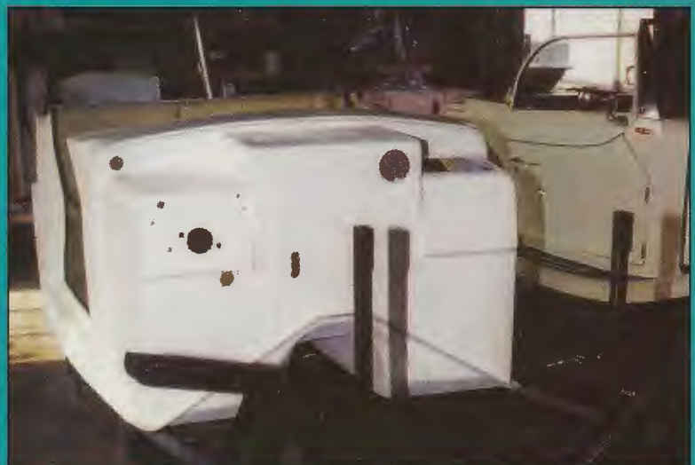
Many of the necessary holes in the front bulkhead are pre-cut at the factory
