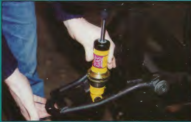
ABOVE: Fabricated wishbones and coil damper units replace the Sierra components.
