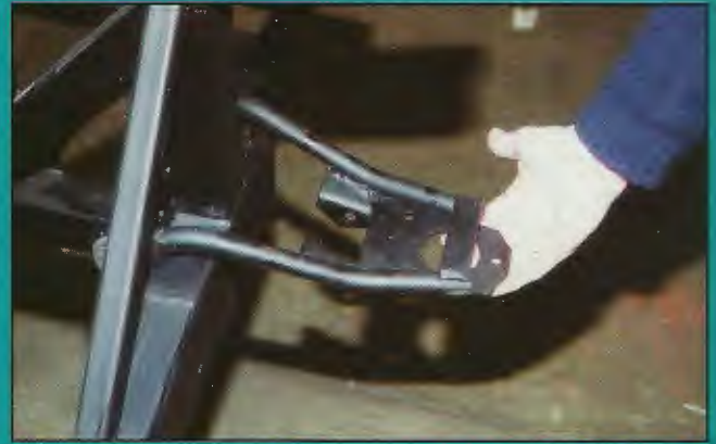
ABOVE: Fabricated wishbones and coil damper units replace the Sierra components.
