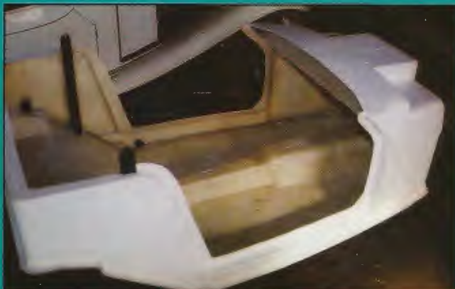
The single-piece main bodytub is fitted to the chassis at the factory. Complete with integral floor that sits on the galvanised steel panelling of the chassis the moulding has cut-outs to take the seat belt mountings shown here on the left of the picture
