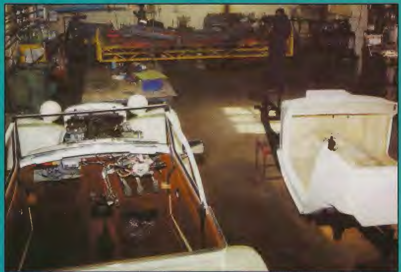
All of the metal fabrication and build work is carried out in the single large workshop - the GRP mouldings are sub-contracted
