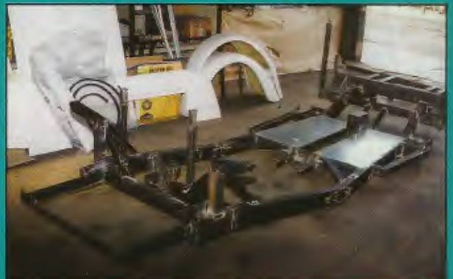
An unpainted chassis sits next to some wings and moulded body parts. Perhaps not the most elegant structure, it is nevertheless very strong and most effective. All the necessary mounting points are incorporated and its final design was the result of much development
